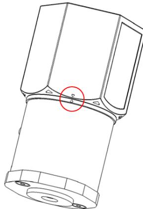
Figure 3.2 Tighten two chassis
