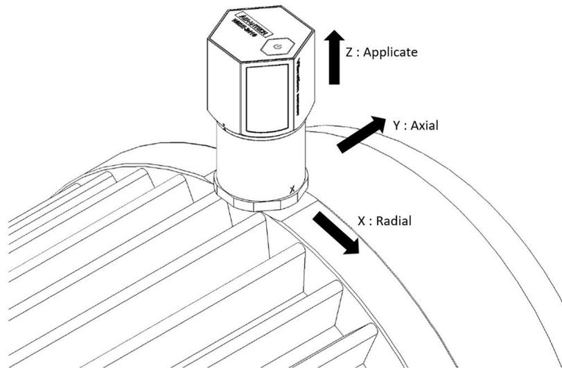
Figure 3.4 WISE-2410 Detail Installation Direction on motor
