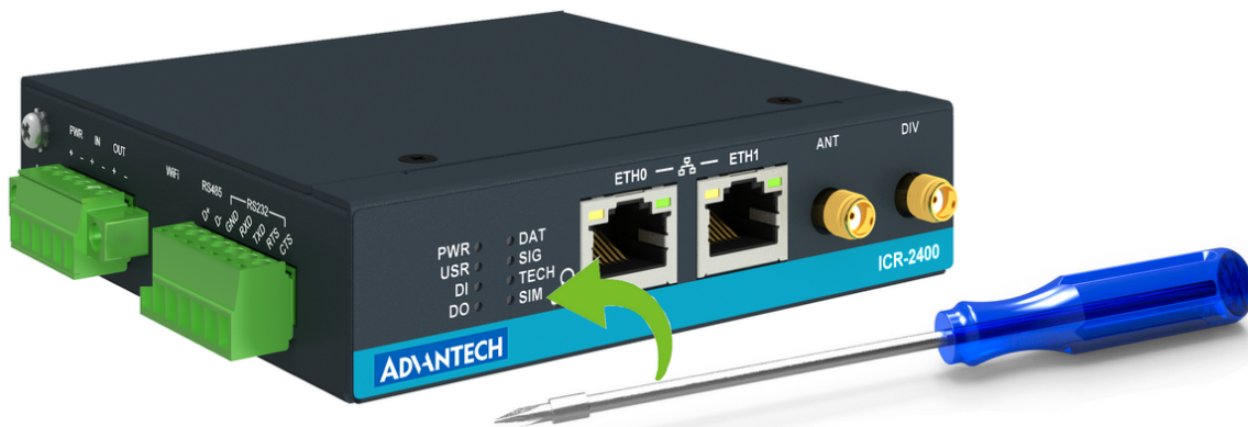
Figure 12: Resetting the Router
