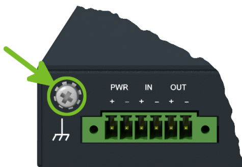
Figure 8: Position of the Grounding Screw
