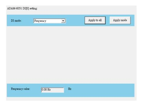
When **Frequency** is selected from the **DI mode** box, the module will calculate the frequency of the digital input signal for the selected channel. This value will be displayed in the **Frequency value** box.
