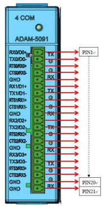
Figure 7.6 ADAM-5091 Application Wiring
