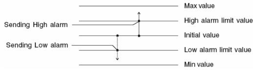
Figure 6.19 Sending Alarm Signal (Recommended Settings)
