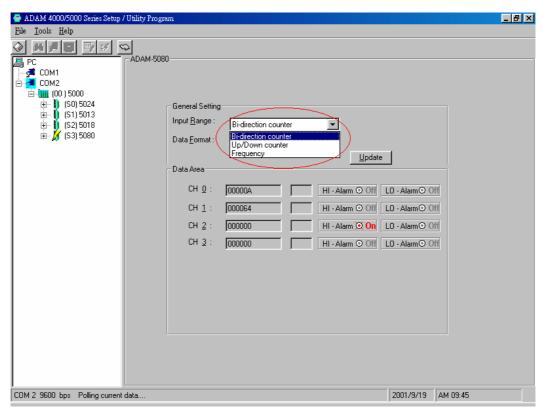
Figure 6.4 Counter / Frequency Mode
