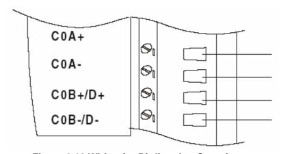
Figure 6.16 Wiring for Bi-direction Counting
