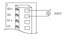
Figure 1.17 Millivolt and Volt Input
