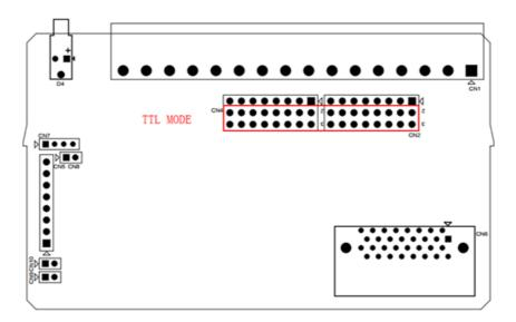
Figure 6.13 Jumper Location for TTL Mode
