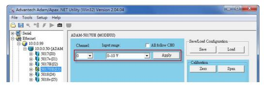
3. Use a precision voltage source to apply a span calibration voltage to the module's V0+ and V0- terminals. (See Tables 5-2 and 5-3 for reference voltages for each range.)
