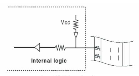
Figure 6.3 TTL Input Level
