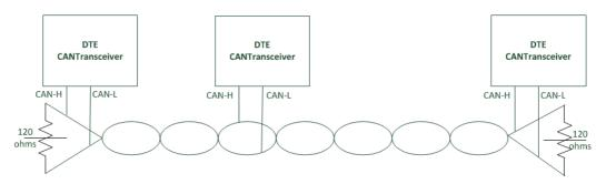
Wiring connections are as follows:
