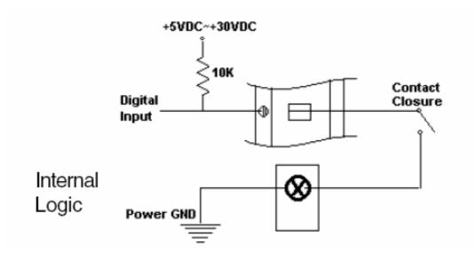
Figure 4.8 Contact Closure Input (ADAM-5051/5051D)
