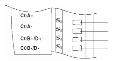
Figure 6.5 Wiring for Up/Down Counting
