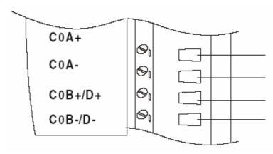
Figure 6.6 Wiring for Bi-direction Counting
