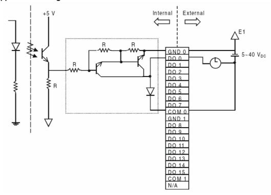
Figure 4.20 ADAM-5056S Module Wiring Diagram
