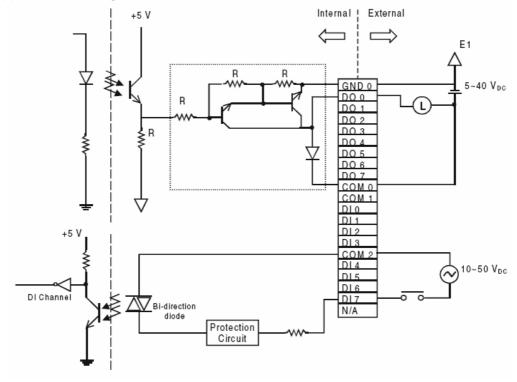
Figure 4.16 ADAM-5055S Module Wiring Diagram
