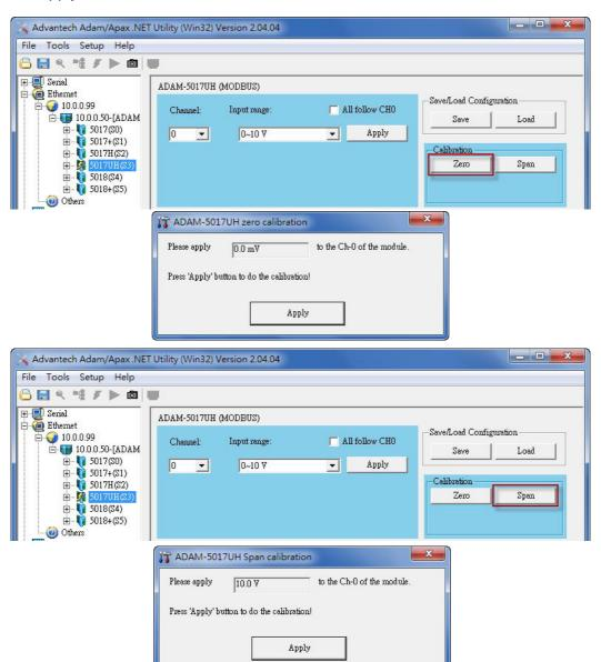
7. Click "Span" and apply the voltage as pop out windows to the Ch-0 and click "Apply."
