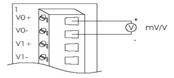
Figure 1.5 Millivolt and Volt Input
