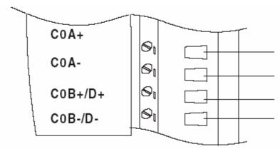
Figure 6.15 Wiring for Up/Down Counting
