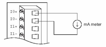
**Figure 3.2 Output Module Calibration**
