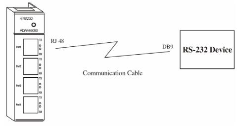
Figure 7.2 ADAM-5090 Application Wiring
