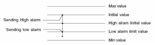
Figure 6.10 Sending Alarm Signal (Not Recommended)
