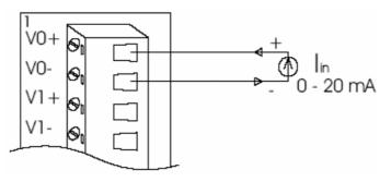
**Figure 1.6 Process Current Input**
