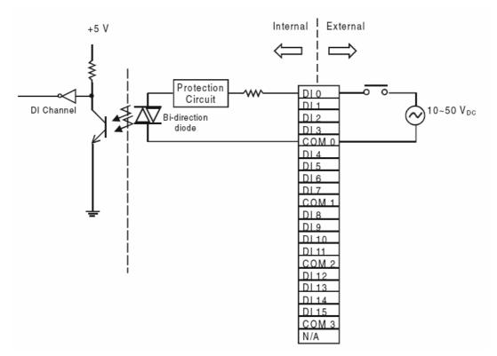
Figure 4.10 ADAM-5051S Module Wiring Diagram
