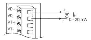
**Figure 1.10 Process Current Input**
