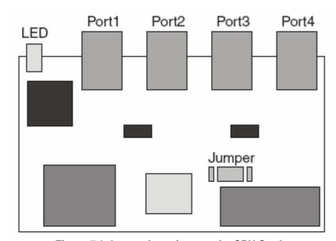
Figure 7.3 Jumper Locations on the CPU Card
