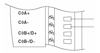
Figure 6.17 Wiring for Frequency Mode
