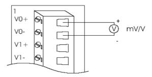
Figure 1.9 Millivolt and Volt Input
