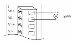
Figure 1.13 Millivolt and Volt Input
