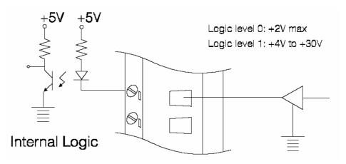
Figure 4.4 Wet Contact Signal Input (ADAM-5050)
