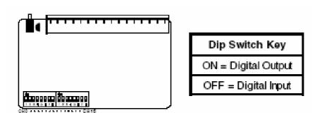
Figure 4.1 DIP Switch Setting for Digital I/O Channel
