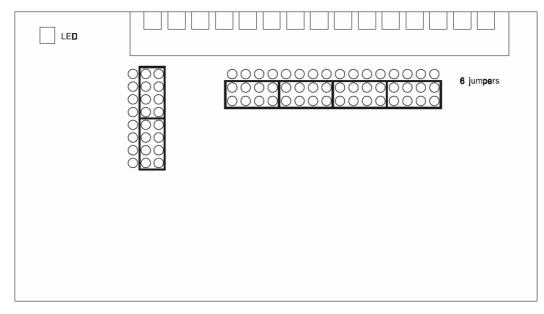
Figure 6.22 Jumper Location on the ADAM-5081 Module
