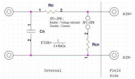
Figure 1.19 Locations of RC Filter Jumper Setting
