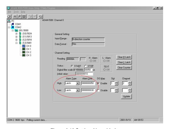
Figure 6.18 Setting Alarm Limit
