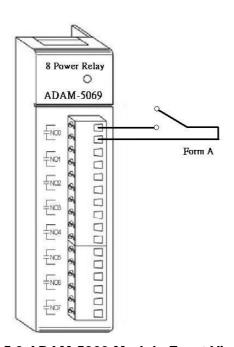
Figure 5.3 ADAM-5069 Module Front View Wiring
