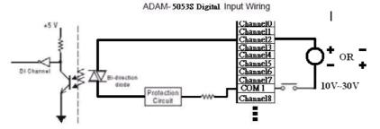
Figure 4.14 ADAM-5053S Module Wiring Diagram
