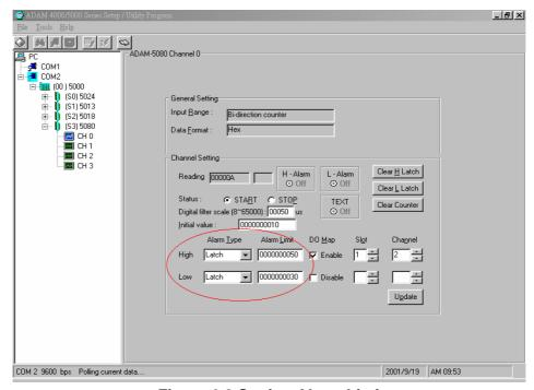
Figure 6.8 Setting Alarm Limit
