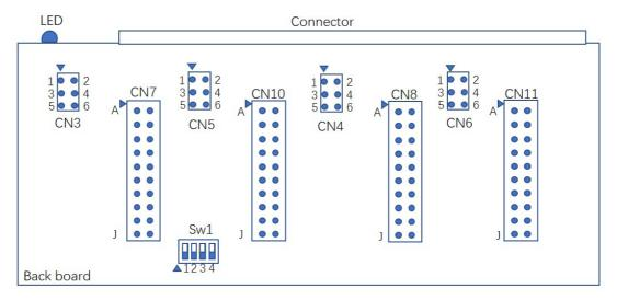
Figure 7.7 ADAM-5091 Jumper and switch location
