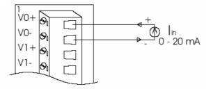
**Figure 1.18 Process Current Input**
