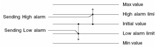
Figure 6.9 Sending Alarm Signal (Recommended Settings)
