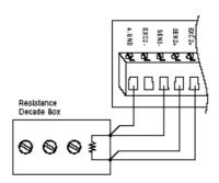
Figure 1.3 Applying Calibration Resistance
