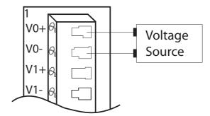
Figure 3.1 Applying Calibration Voltage
