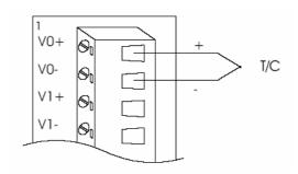
Figure 1.24 Thermocouple Input
