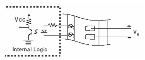
Figure 6.2 Isolated Input Level
