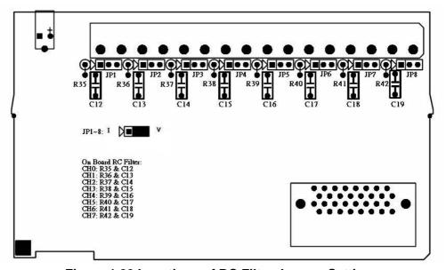
Figure 1.20 Locations of RC Filter Jumper Setting
