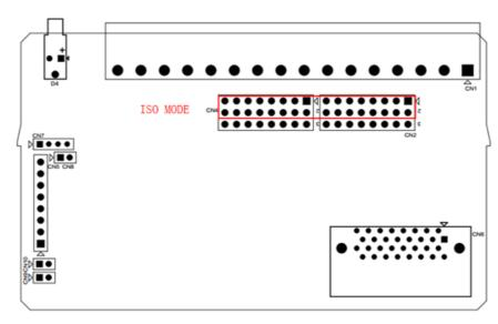
Figure 6.12 Jumper Location for Isolation Mode
