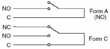
Figure 5.2 Relay Output
