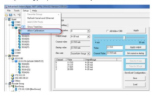
Connect either a 5-digit mA meter or voltmeter with a shunt resistor (250 ohms, .01 % and 10 ppm) to the screw terminals of the module.
