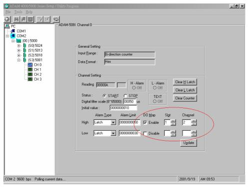
Figure 6.21 Digital Output Mapping
