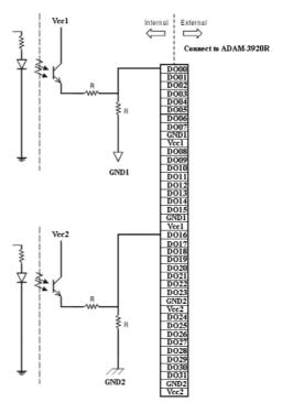
Figure 4.24 ADAM-5057S Module Wiring Diagram
