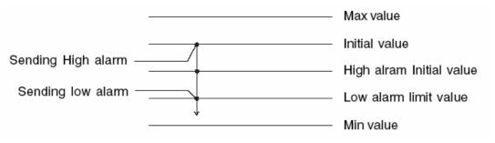
Figure 6.20 Sending Alarm Signal (Not Recommended)
