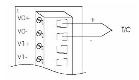
Figure 1.22 Thermocouple Input
