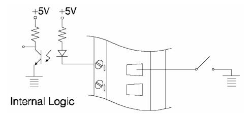
Figure 4.3 Dry Contact Signal Input (ADAM-5050)
