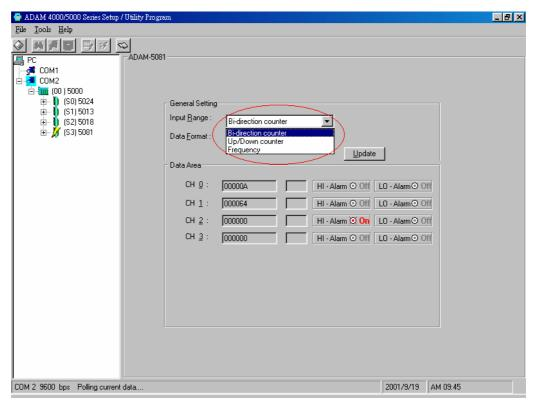
Figure 6.14 Counter / Frequency Mode
