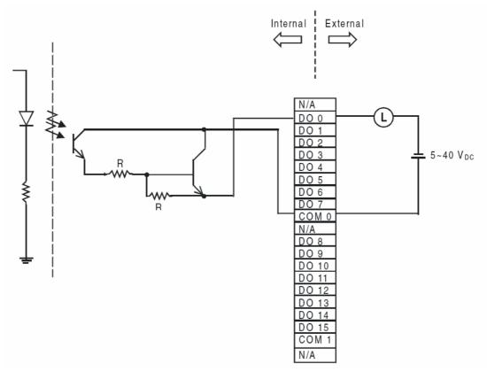
Figure 4.22 ADAM-5056SO Module Wiring Diagram
