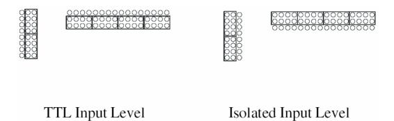
Figure 6.23 TTL/Isolated Input Level Select
