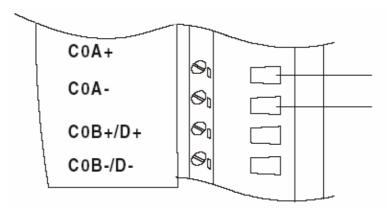
Figure 6.7 Wiring for Frequency Mode
