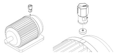
Figure 3.8 Adhesive Mounting Pad
