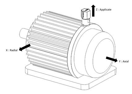
Figure 3.3 WISE-2410 Installation Direction on motor
