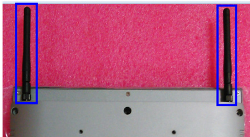
Figure 2.21 Location of external antennae
