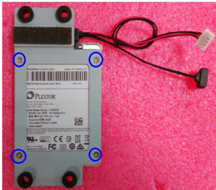
Figure 2.11 Secure SATA HDD with screws
