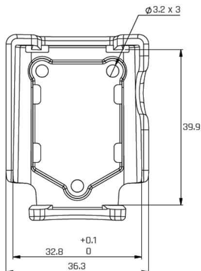
Figure 4: Clip (without device) – front view
