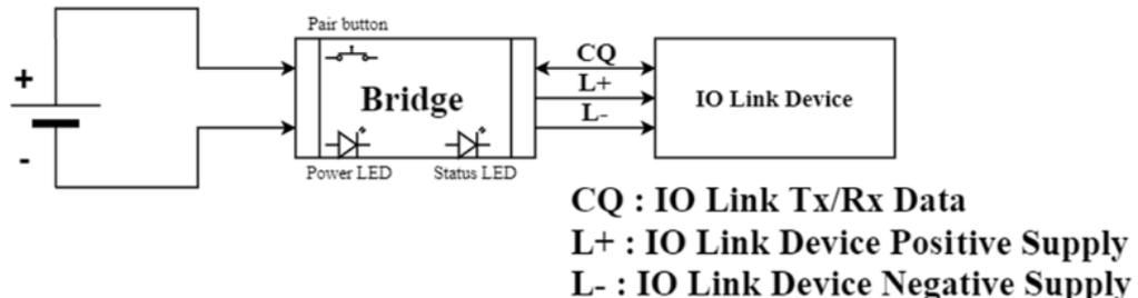
Figure 7: Connection of the IO-Link Device to the Wireless Bridge (block diagram)
