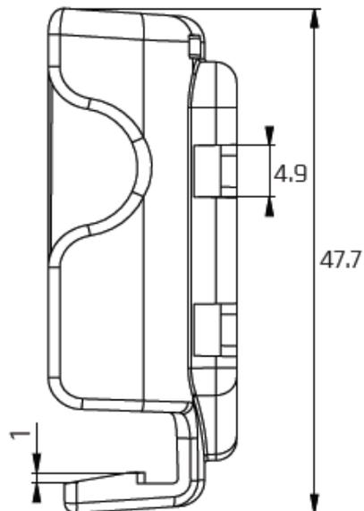
Figure 5: Clip (without device) - side view
