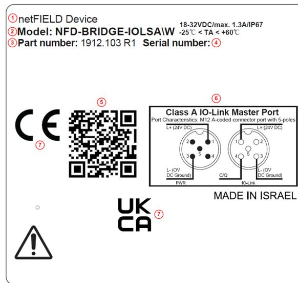
Figure 2: Device label Wireless Bridge NFD-BRIDGE-IOLSAIW
