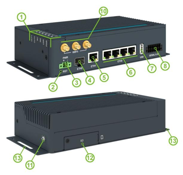
Figure 5: Hardware Overview of the Router
