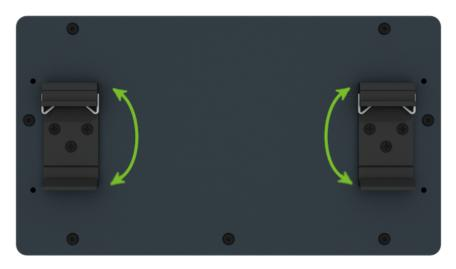
Figure 8: Default Position of the DIN Rail Clips
