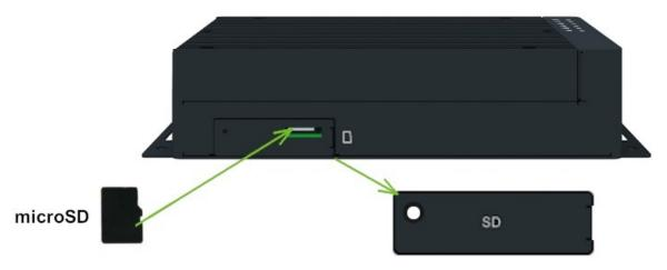
Figure 13: MicroSD Card Insertion
