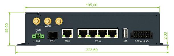
Figure 5: Router Dimensions - Front View
