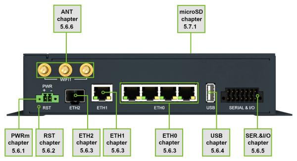
Figure 15: Router Connection
