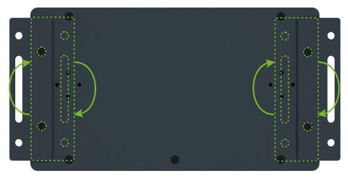
Figure 7: Rotated Wall Mounting Clips
