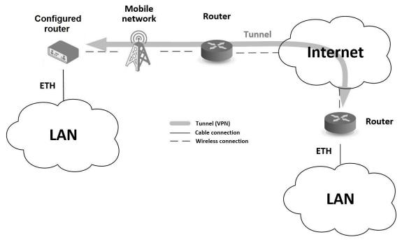
Figure 3: Using VPN Tunnel
