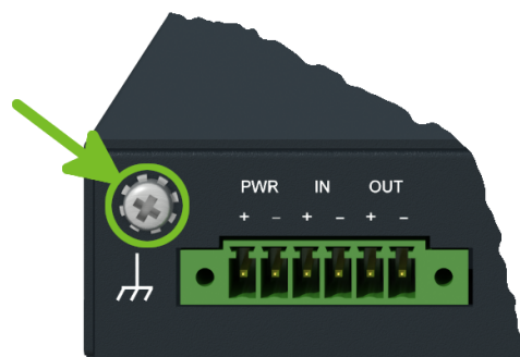
Figure 8: Position of the Grounding Screw
