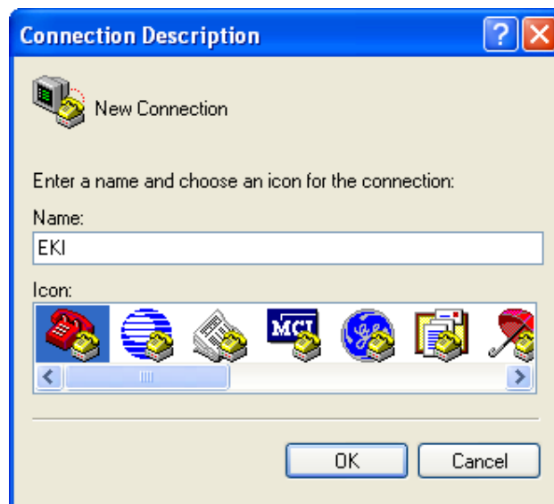
Figure 7.1 Creating a Telnet Connection
