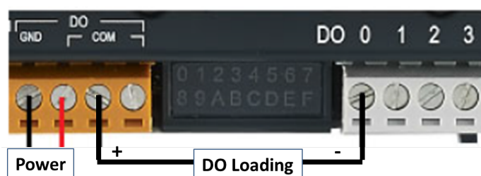
Figure 3.4 Digital Output Wiring
