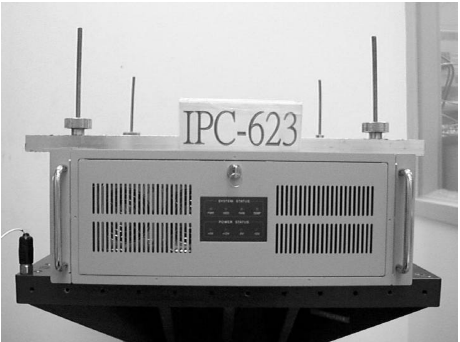
The IPC-623 Z axis random vibration test
