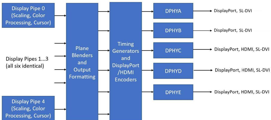
**Note:** Do not design with HDMI™ connector on Port A or B.
