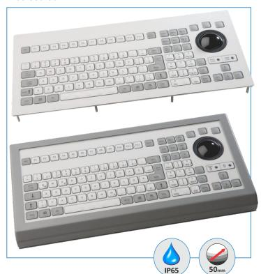
The unit features a full MF (multi-functional) keyboard with separate numeric-, cursor- and control keypads. The large, robust industrial grade trackball has a ball diameter of 50 mm and allows highest precision in cursor control. The keyboard part is sealed to IP65, the self-adjusting PTFE seal of the trackball enables an IP65 static (ball in rest) protection grade. Colour scheme and legend styling fit with the most recent industrial computer equipment.
