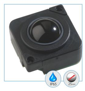
The GK25 features a phenolic ball with metal core, stainless steel shafts and bearings for a smooth and precise cursor control. The PTFE seal ring ensures a IP65 static sealing grade. The unit has been designed to be back of panel mounted as part of OEM keyboards and consoles with restricted mounting space.
