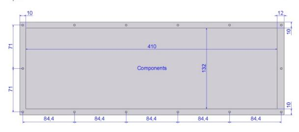
COLOURS Keyboard Background : RAL7035 Light grey Key Background : RAL9010 Pure white Key edges & legends : RAL5003 Sapphire blue Enclosure : RAL7037 Dusty grey Dim in mm
