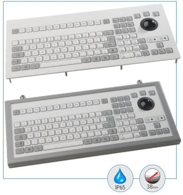
The unit features a full MF (multi-functional) keyboard with separate numeric-, cursor- and control keypads. The robust industrial grade trackball has a ball diameter of 38 mm and allows highest precision in cursor control. The keyboard part is sealed to IP65, the self-adjusting PTFE seal of the trackball enables an IP65 static (ball in rest) protection grade. Colour scheme and legend styling fit with the most recent industrial computer equipment.
