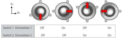
Figure.1 Mounting Orientations
