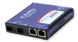
The IE-MultiWay is a value-based, Carrier-class managed Gigabit Ethernet solution that is ideal for use as a CPE device at the customer's network edge as well as in a fiber infrastructure. The IE-MultiWay comes standard with two SFP ports for the providers' network connection and two fixed 10/100/1000Base-T copper ports. There are four distinct DIP Switch selectable configurations that the IE-MultiWay supports.
