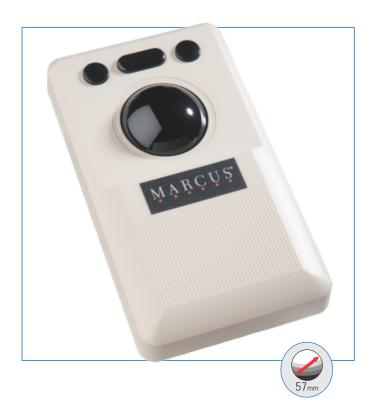
The R55 is a professional desk top trackerball. This trackerball is designed for comfort over prolonged periods of use. Constructed from high impact plastic and featuring robust mechanics, it is ideally suited for use where reliability and an extensive live span are prerequisites. The unit is directly connectable to any PC USB mouse port or to a PS/2 port via the supplied USB to PS/2 adaptor. No special device driver is required.
