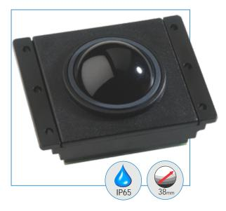
The GK38 series are ruggedised professional trackballs for harsh industrial environments. The double-sided seal ring provides a sealing to IP65 static (ball in rest). Stainless steel shafts and bearings ensure a solid and precise pointer control. The unit can be used for frontpanel mounting (remove the mounting bracket) or for backpanel mounting.
