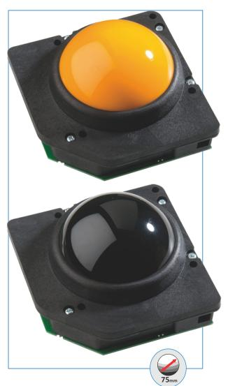
The GK75 is a very high specification, back of panel mounted trackball with large 75 mm ball diameter. It is constructed from PPS and benefits from its large diameter shafts and bearings for smooth running. It is designed to be rear-panel mounted as part of OEM systems, where reliability, robustness and an extensive life span are essential. The large ball provides the perfect solution for high performance, high resolution applications.
