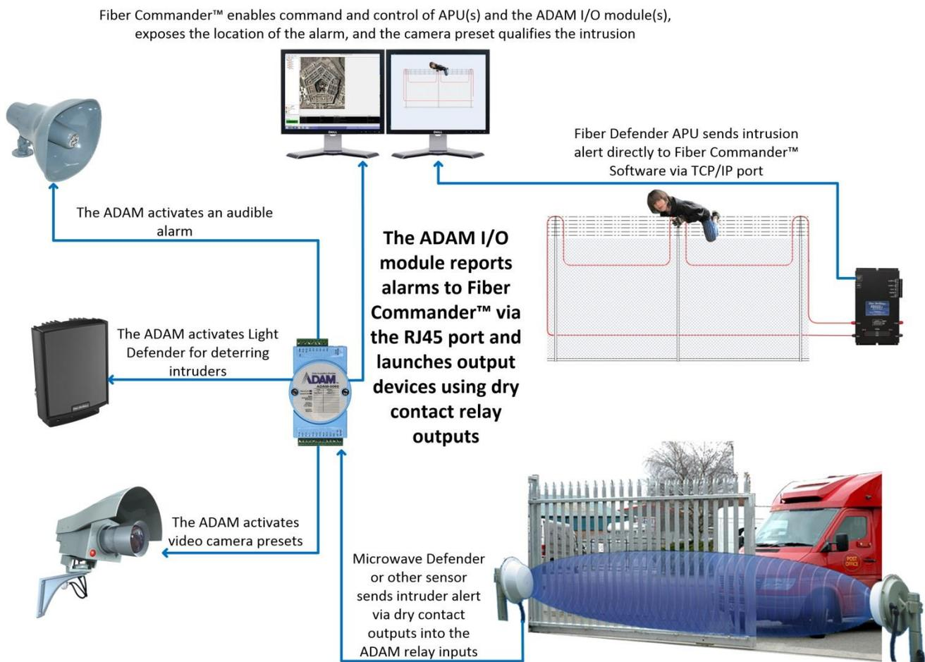
**Picture 2: The ADAM Module and Fiber Commander Head End Software, connected to multiple devices**
